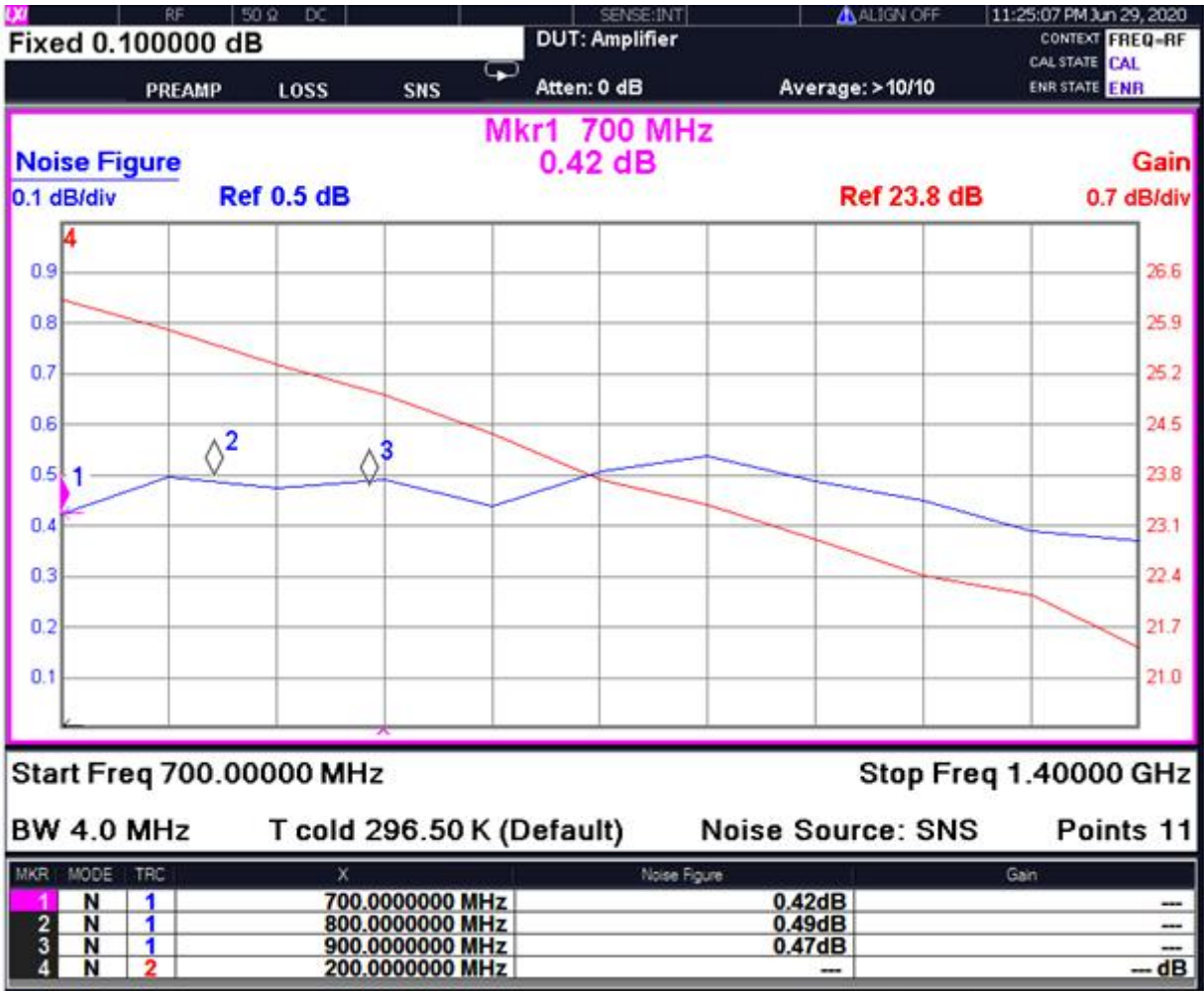
Evaluation Board NF, Gain, and Return Losses for 700 to 1000 MHz Tuning
