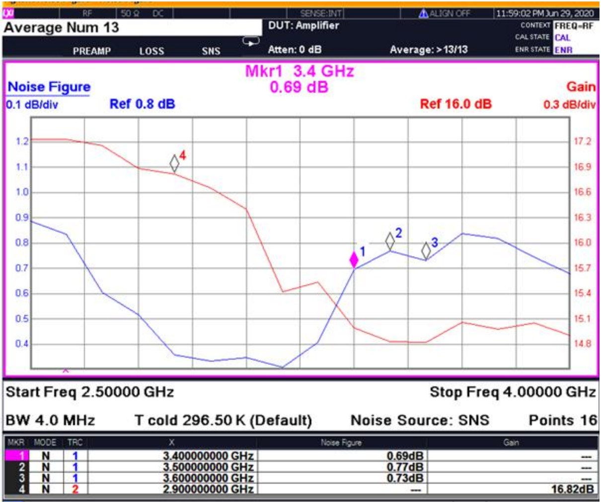
Evaluation Board NF, Gain, and Return Losses for 3.3 to 4.0 GHz Tuning
